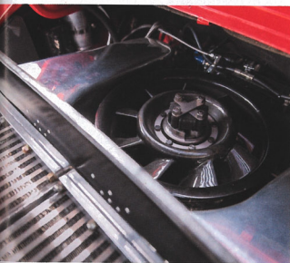
BELOW 962's horizontal cooling fan position is retained
